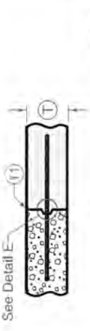
'KT' ABUTTING PAVEMENT JOINT - KEYWAY TIE
